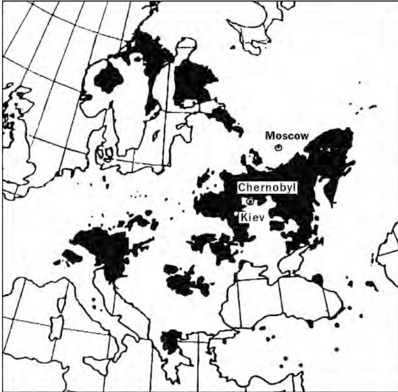
Figure 1.6. Some of the main areas of Europe contaminated at a level higher than 1 Ci/km 2 by Cs-137 as a result of the Chernobyl catastrophe. Turkey was surveyed only in part and Bulgaria, Yugoslavia, Portugal, Iceland, and Sicily were not surveyed at all (Cort and Tsaturov, 1998).
